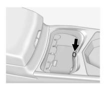
This vehicle has a cupholder equipped with a divider that can be adjusted to accommodate large containers or small containers.
